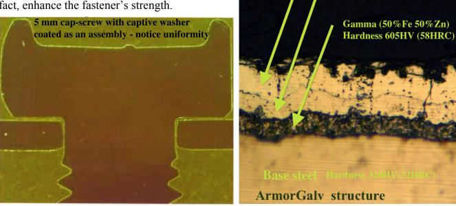
As can be seen from the above cross section of a screw, the ArmorGalv layer is very uniform, precise and controlled.
