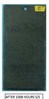
The salt spray testing was stopped at 1,008 hours with no signs of red rust.
