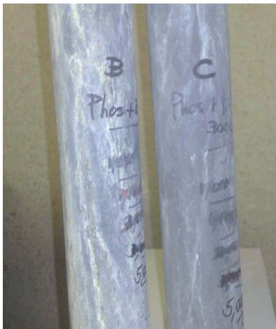
ArmorGalv® Natural 400 microns, 5000-hour B117 salt spray.
