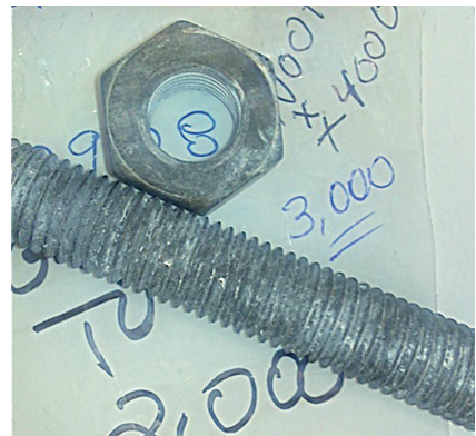
ArmorGalv® Bronze 25 microns, 4000 hr. B117 salt spray.
