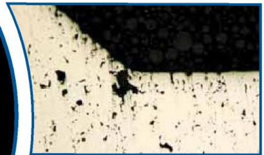
Powder Metal Parts Before ArmorGalv®
