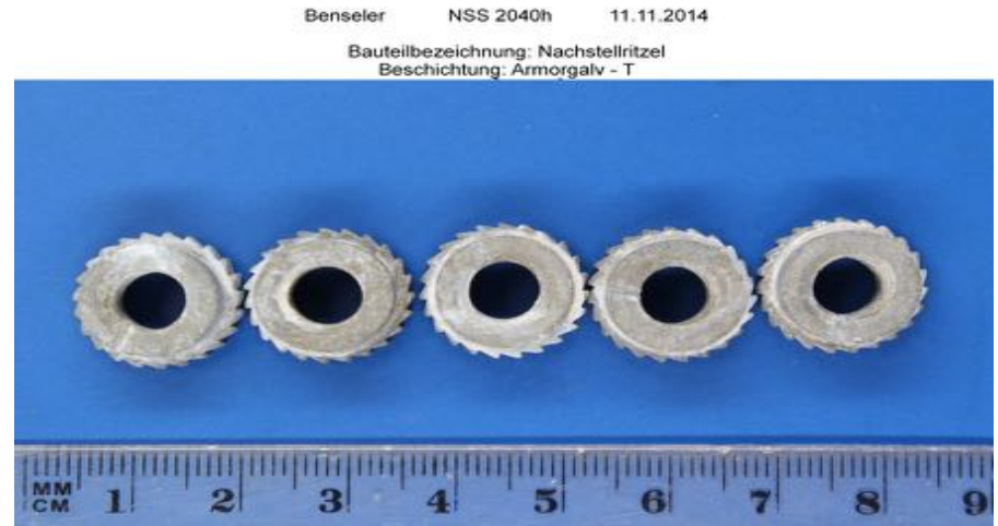
Sintered steel ratchet wheels (2040 Hrs salt spray)
