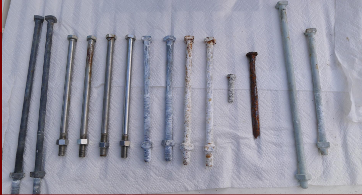
From left to right: TDG (2), 316 SS (2), 304 SS (2), Silicate Coated HDG (2), HDG (2), Aluminum (1), electroplated (1), ERX TDG (1), ERX HDG (1)
