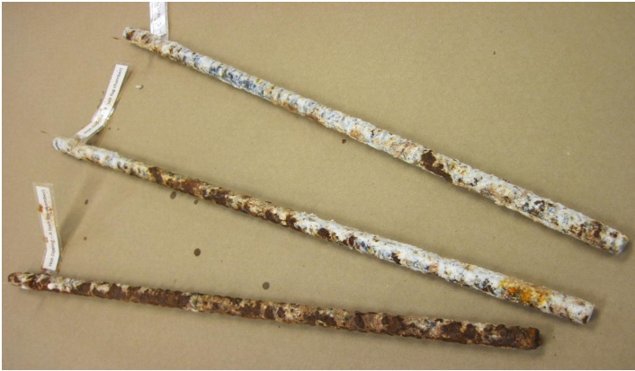
Figure 3 Traditional Hot Dipped galvanizing after 3000 hours in salt fog exposure
