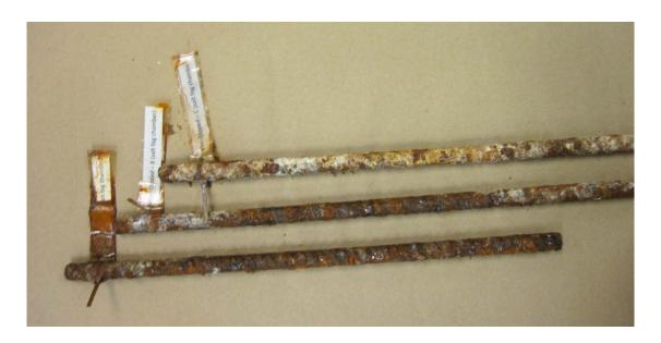
Figure 3 Traditional Hot Dipped galvanizing after 10,700 hours in salt fog exposure
