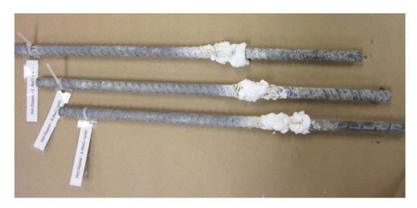
Figure 1 Traditional Hot Dipped galvanizing after 10,700 hours partial immersion
