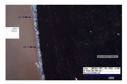
Figure 5 Unexposed specimen of ArmorGalv  $^{\circledR}$
