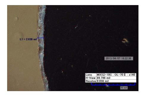
Figure 6 ArmorGalv® after 3000 hours in salt fog environment
