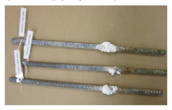
Figure 2  $\,$  Armorgalv $^{\textcircled{\tiny{\$}}}$  process after 10,700 hours of partial immersion
