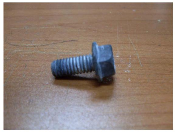
The results of an evaluation of the coating system of sample bolt Daetwyler Clean Energy 500402495 demonstrated that it provided protection at least equivalent to that provided by the zinc coating as described (ASTM G90) in 10.2(a).
