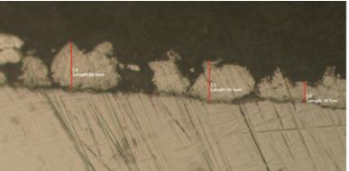
Total Thickness: Inch n/a μm 31.50 Magnification: 200X
