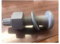
The coating "looks good" uniform with full coverage, and magnetic thickness testing indicates a  $30\mu$  result. But predicting how well this coating will actually perform can only be definitively ascertained by peering into what lurks below the surface, a skill a met lab technician only shares with Superman.
