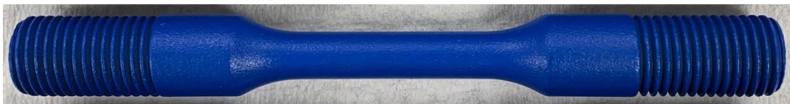
Figure 2: Test specimen with Coating A (1.5-2 mil total TDZ & 1 mil Armorplex) before exposure.
