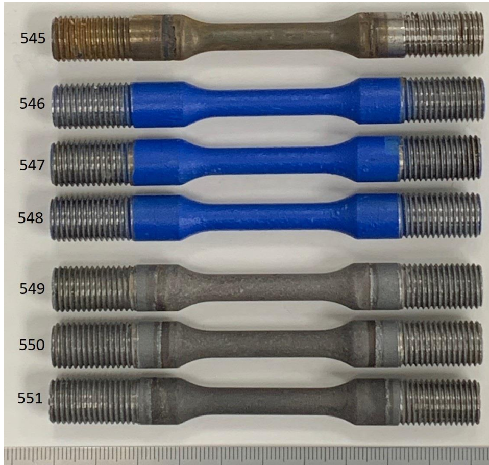
Figure 8: Test specimens after the 720-hour exposure in environment 1.
