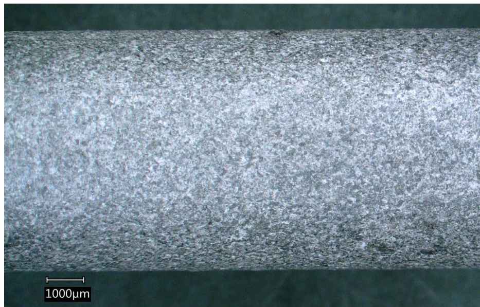
Figure 11: Test specimen 549 with Coating B (1.5-2 mil total TDZ & 1 mil Sealer only) after exposure in environment 1, at 20X magnification.
