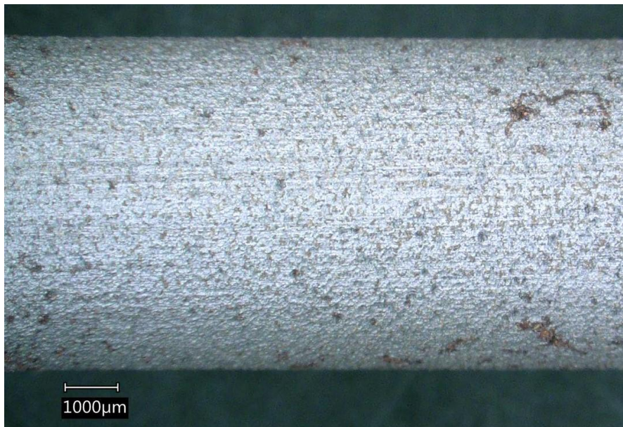
Figure 13: Test specimen 556 with Coating B (1.5-2 mil total TDZ & 1 mil Sealer only) after exposure in environment 2, at 20X magnification.
