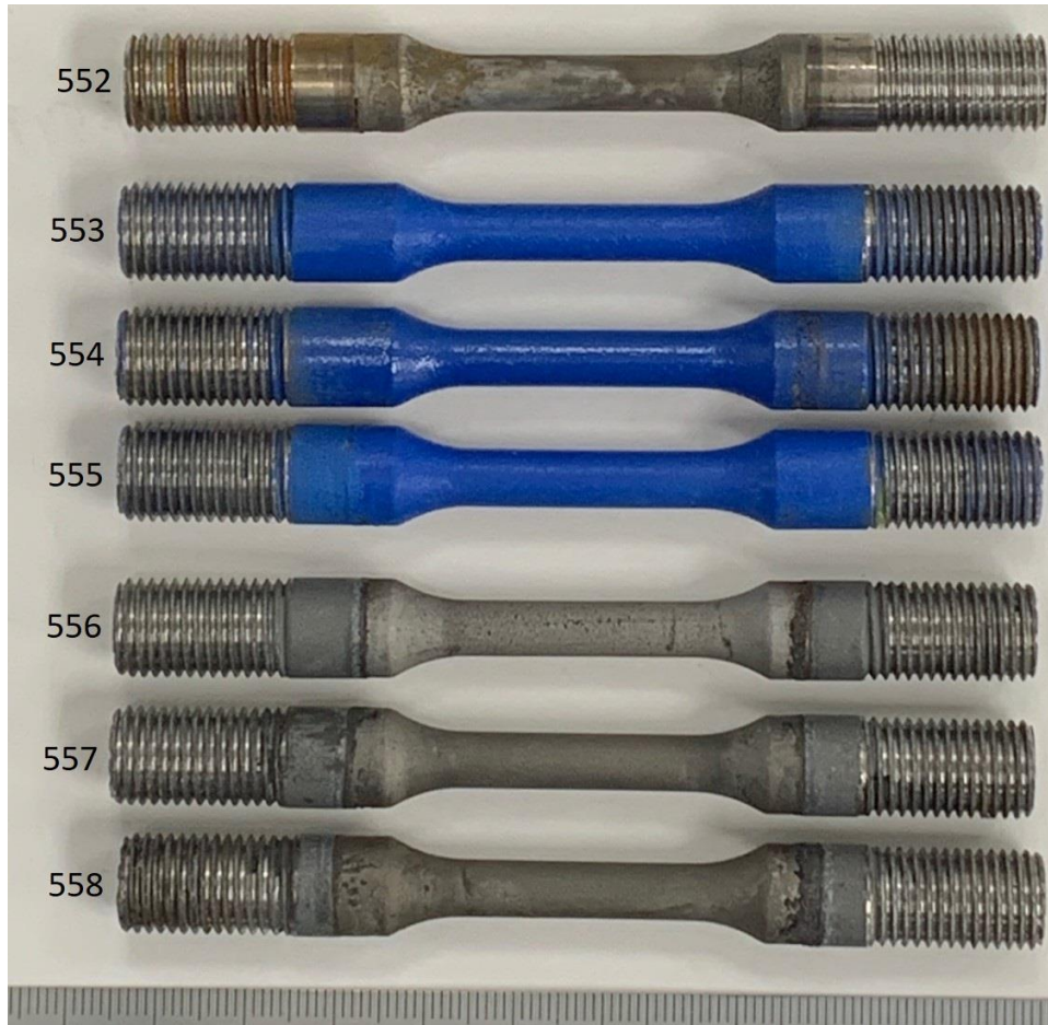
Figure 9: Test specimens after the 720-hour exposure in environment 2.
