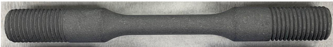
Figure 3: Test specimen with Coating B (1.5-2 mil total TDZ & 1 mil Sealer only) before exposure.
