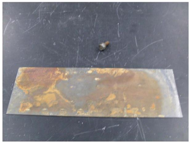
Both the sample and control were washed in DI water to remove oxide reside. The sample bolt was compared to the control plate (both sides and scribed area).
