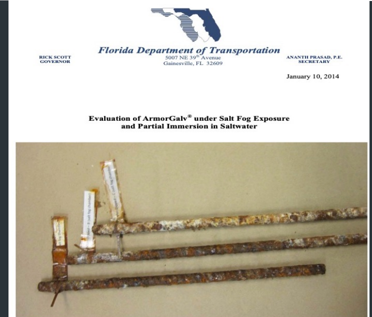
Figure 3 Traditional Hot Dipped galvanizing after 10,700 hours in salt fog exposure
