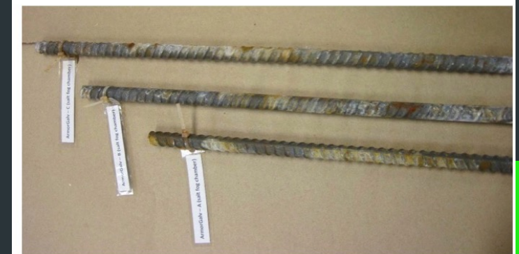
Figure 4 Armorgalv ® process after 10,700 hours in salt fog exposure
