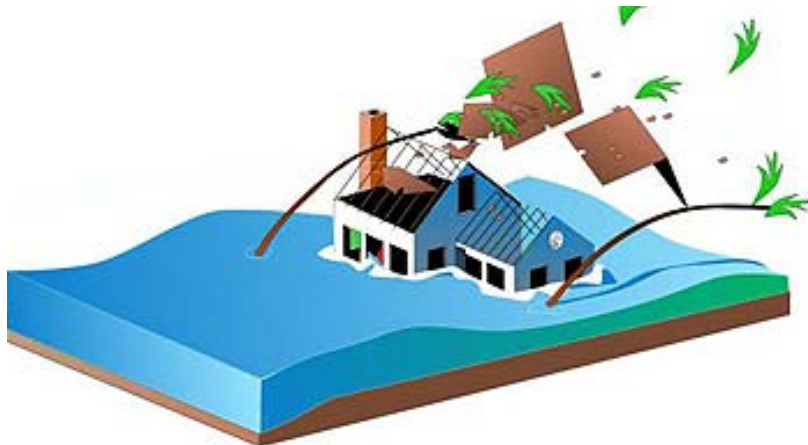
This is what happens in a storm, if fasteners corrode and no longer have the holding power required to hold the roof in place.
